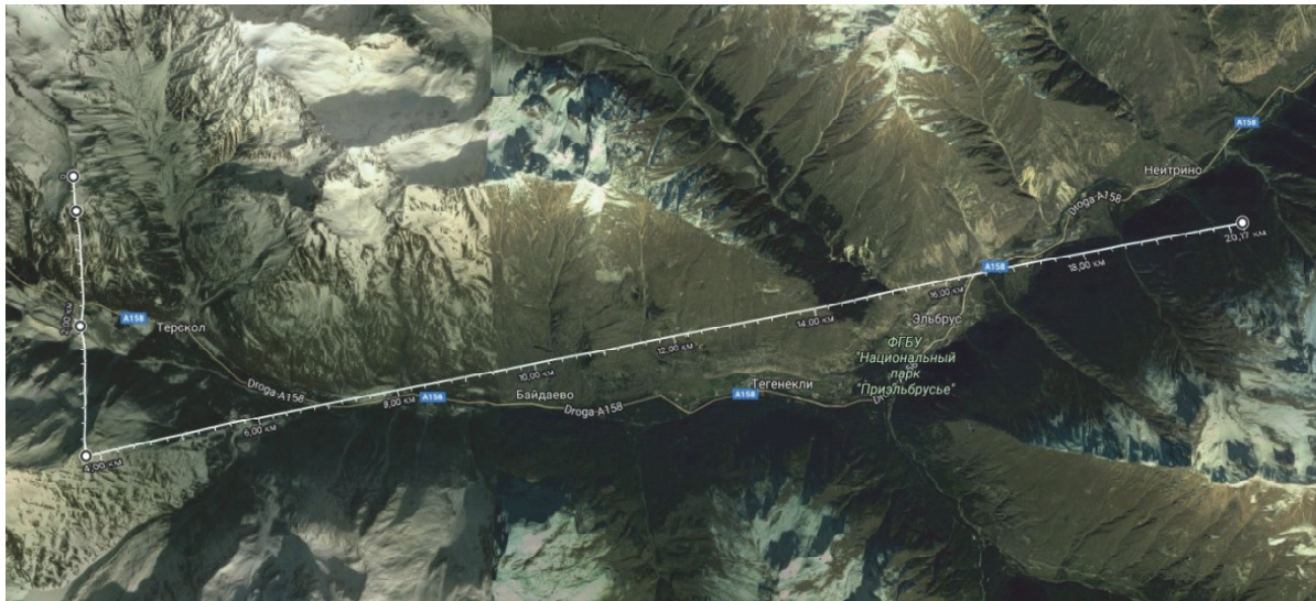
Fig1. Scheme of networking. The local networks of BNO and Terskol Peak Observatory are joined by means of radiochannel implemented on three Cisco Aironet 1410 modules. One module operates at Cheget peak in the access point mode. Two others modules operate in bridge mode at the «Andyrchy» EAS array and at the Terskol peak.
